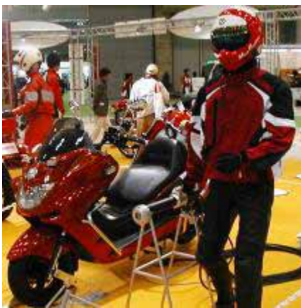
Firefighting motorcycle: The mannequin is holding a water jet nozzle (slightly below the center of the photo).
