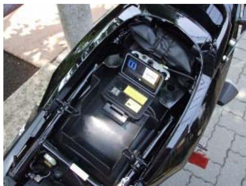
Onboard unit housed under the seat.
